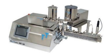
Twin screw laboratory extruder ZE 12 HMI
