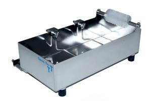
The cooling bath in different lengths and designs is used for efficient cooling of various extrudates before further processing by means of a winder or pelletizer. It is equipped with holding-down bars or holding-down rollers and scraper brush and mounted on damping elements. The water can be drained via a valve. In our larger cooling baths, a cooling unit can be connected and the water level is adjustable.
