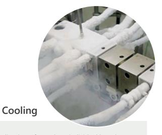
Cooling is performed per individual barrel zone. It is possible to operate the cooling manually or to regulate it via the extruder control system using solenoid valves. Water cooling, air cooling or liquid nitrogen cooling are available.
