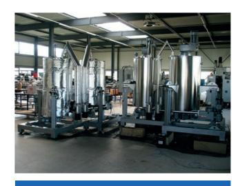
Battery production feeding systems completely insulated
