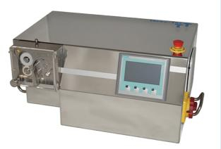
The pelletizer can be used to process strands into pellets or granules. The speed of the feed roller and the cutter are independently adjustable. This allows the extrudate feed to be perfectly matched to the extrudate and the pellet length or pellet size to be adjusted between 0.5 and 10 mm during
