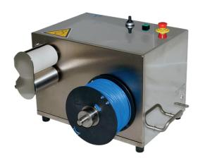
The filament winder from Three-Tec is suitable for winding the extrudate onto a spool. The tensile force between the take-off roller and the spool is adjustable, which enables very uniform winding. In addition to round strands, the winder can also be used to wind ribbon-shaped extrudates onto a spool. The filament winder is controlled by means of an integrated potentiometer.
