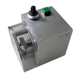
With the hot cutter, the extrudate can be reliably processed into pellets or granules with one or more knives in direct contact with the die plate. Both wet and melt extrudates can be processed. The number of knives used and the speed setting allow the production of pellet lengths or pellet sizes between 0.5 and 10 mm.
