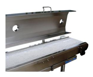
The cooling conveyor belt is suitable for the gentle removal and efficient cooling of extrudates and granules. The conveyor belt rests on actively cooled cooling elements and is permanently cooled during operation. Air connections in the lid of the cooling conveyor belt allows additional air cooling of the product. The belt speed can be variably adjusted between 0 and 20 m/min.
