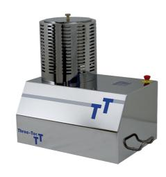
The Spheronizer is used for reducing the length and rounding off fine extrudate strands. The desired geometry of the end product is influenced by the batch size, the speed and
