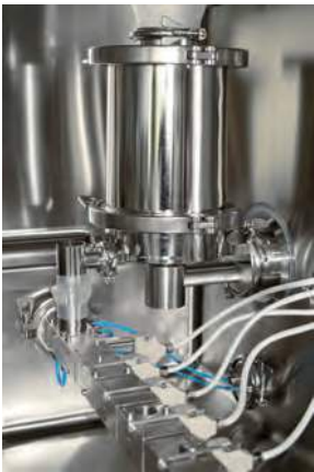
integrated in the isolator are made of stainless steel 1.4404 (316 L) with a surface finish of Ra \leq 0.8 \mu m .
